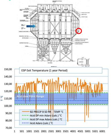
→ Due to combustion of particular imported coals the flue gas temp. is critically close to the acid dew point and in some periods bellow it
